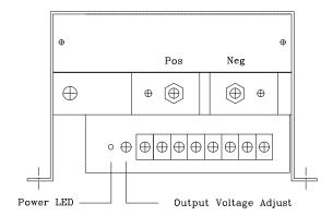
The 1939SM is a 32 amps, 500 watt switch mode power supply.
